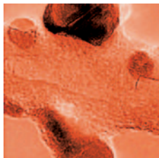
TEM image showing the polymer interlayer between silver nanoparticle and nanotube wall Chao Gao et al 2006 Nanotechnology 17 2882–2890
